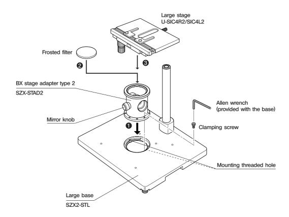
★ For simplified transmitted light observation, place the mirror knob on the front and use a frosted filter.
