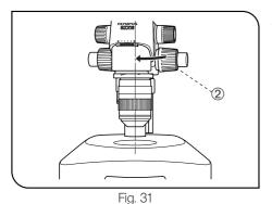
2. Return the microscope body to the illumination light path by loosening the focusing module clamping knob ②, rotating the microscope body gently in the direction of the arrow, aligning visually the objective with the illumination light path and tightening the clamping knob ② again.
