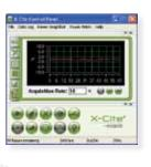
A custom graphical user-interface (GUI) enables computer control of all X-Cite® exacte functions, logs events and records and displays real-time stability data. Ideal for verifying intensity stability during automated or long term imaging experiments.
